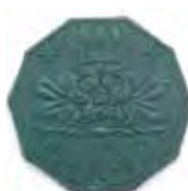
A rubber positive representation of the reverse of the George VI CD; one of the several steps in the process to make the die that will strike the medals. Most of these steps are no longer necessary thanks to modern technology.
